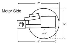
Motor: .06 amp, 60Hz 110v 1ph 6 rpm continuous duty.
